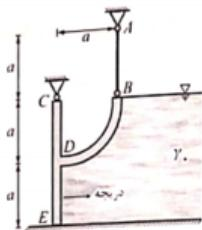
$$\left\{ \begin{array}{l} \sqrt{Mc} = 0 \longrightarrow F_{AB} \times a + F_y \times \frac{4a}{3\pi} = F_X \times \frac{2}{3}(2a) \\ F_V = \gamma V = \gamma_o \times \frac{1}{4}\pi a^2 \times 1 = \frac{\pi}{4}\gamma_o a^2 \\ F_X = \gamma \bar{h}A = \gamma_o \times a \times (2a \times 1) = 2\gamma_o a^2 \end{array} \right.$$
