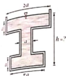
$$\left. \begin{array}{l} F = P \cdot A \\ P = \gamma h \end{array} \right] \longrightarrow F = \gamma h A \quad W = \gamma V$$
