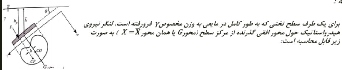
$$\left. \begin{array}{l} M = F \times d = F \times (y_p - \bar{y}) \\ F = \gamma \bar{h} A \\ y_p = \bar{y} + \frac{Ig \sin^2 \theta}{\bar{h} A} \end{array} \right\} \rightarrow M = \gamma \bar{h} A \left( \frac{Ig \sin \theta}{\bar{h} A} \right)$$
