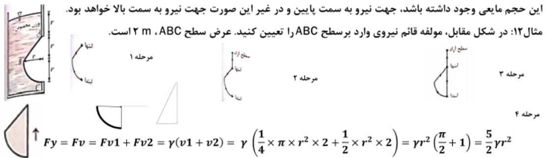
$$F_y = Fv = Fv_1 + Fv_2 = \gamma(v_1 + v_2) = \gamma \left( \frac{1}{4} \times \pi \times r^2 \times 2 + \frac{1}{2} \times r^2 \times 2 \right) = \gamma r^2 \left( \frac{\pi}{2} + 1 \right) = \frac{5}{2} \gamma r^2$$
