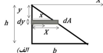
$$F = \int P \, dA = \int_0^h (\gamma y) \left( \frac{yb}{h} dy \right) = \frac{\gamma b}{h} \int_0^h y^2 dy = \frac{\gamma b}{h} \left( \frac{y^3}{3} \right)_0^h = \frac{1}{3} \gamma b h^2$$
