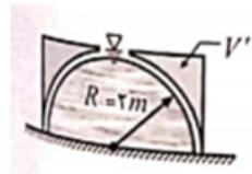
$$F_V = \gamma V, \quad V = V - V_{\text{نیم کره}} = \pi R^2 \times R - \frac{2}{3}\pi R^3 = \frac{\pi R^3}{3} = \frac{\pi \times 2^3}{3} = 8$$
