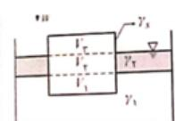
$$FB = \gamma_1 V_1 + \gamma_2 V_2$$
